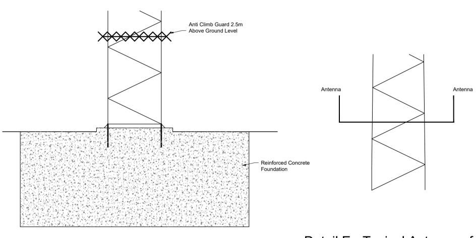
Detail D - Typical Mast Base Detail Scale 1:50
