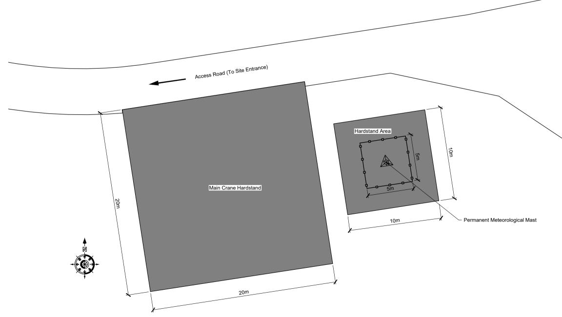
Permanent Meteorological Mast Layout Scale 1:200
